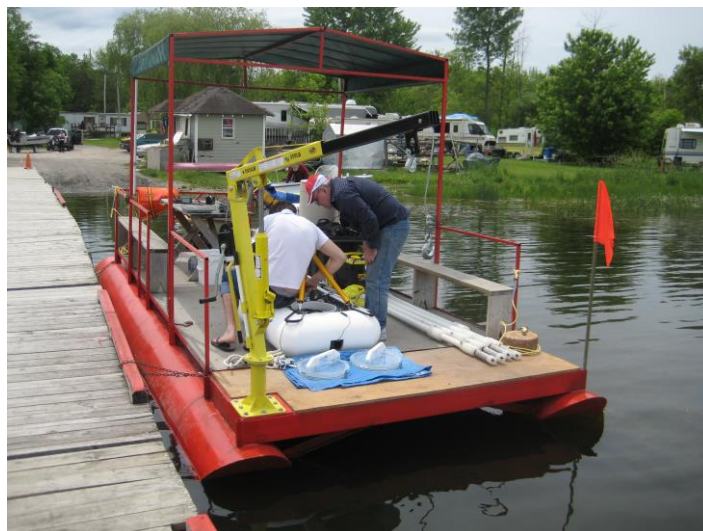
Figure 3 2-channel EM receiver for transition zones SMMT. Preparations for the deployment on the deck of the pontoon boat.
