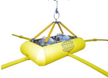
Figure 2: Marine EM receivers for transition zone exploration; 2-channel SMMT.
