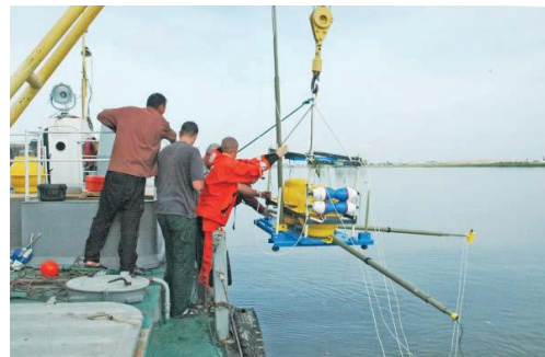
Figure 5: Nord West Ltd. (Moscow, Russia) personnel deploy a shallow-water Marine MT system in the Caspian Sea.
