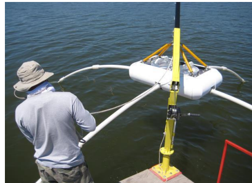
Figure 3: Deployment of SMMT system during marine EM survey from the pontoon boat.
