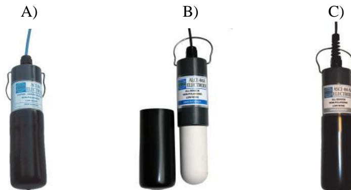
Figure 2: Low-noise non-polarizing electrodes; A) ACE-84 (copper); B) ALCE-84A (lead); C) ASCE-84AG (silver).
