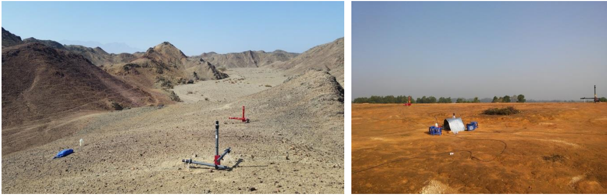
Figure 5 Application of broadband multifunction EM instruments for data acquisition with AMT, MT, BMT, MVP and TC methods.
