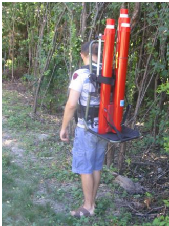
Figure 1: Typical layout of MVP (with AMT) observation site in the field; A) - tripod with magnetic sensors in data record mode; B) - typical 5-component AMT/MVP site layout; C) - tripod in transportation mode.
